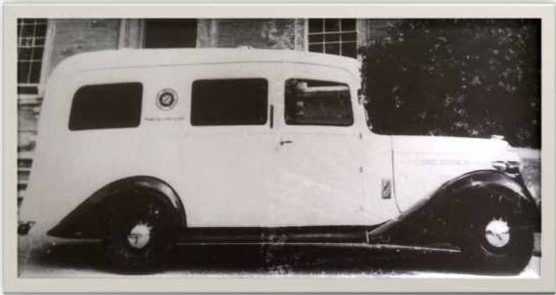
A Grose bodied ambulance for St John Ambulance Brigade on 1939 25hp Vauxhall chassis, based at the Margaret Spencer Convalescent Home in Dallington.
